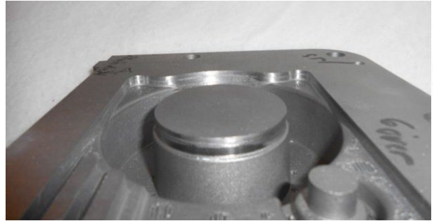
Figure 23. Titanium mold post edge polishing.
