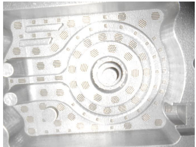
Figure 20. Overall view depicting small vents in difficult locations.
