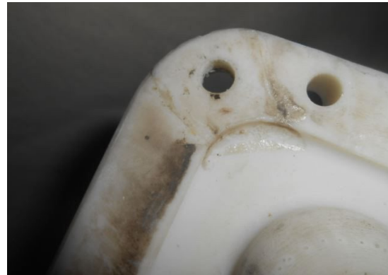
Figure 43. Chipping around the ceramic mold mounting hole and glue repair.
