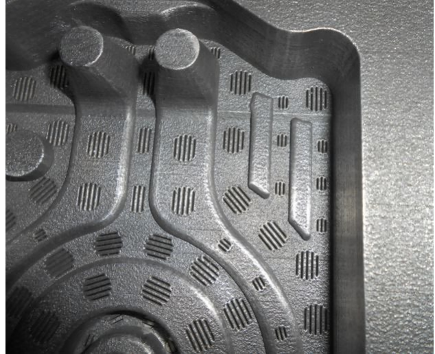
Figure 19. Installation of vents in tight corners using DLS.
