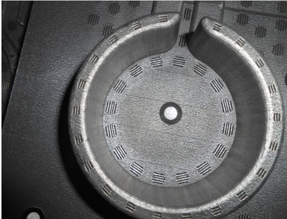
Figure 17. Polished bore ID to reduce faceting and microvent view on the bore top edge.
