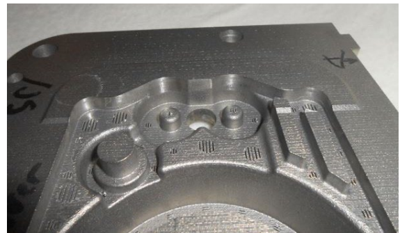
Figures 25. Ti mold vertical wall polishing.
