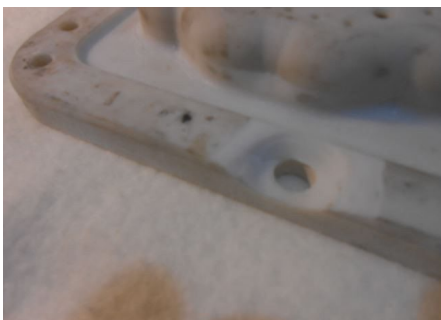
Figure 40. Chipping around the ceramic mold mounting hole.
