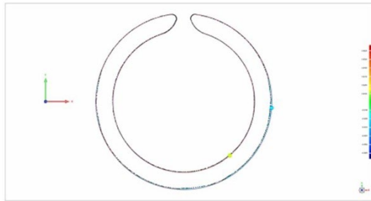
Figure 9. Barrel faceting caused by file export fineness setting.
