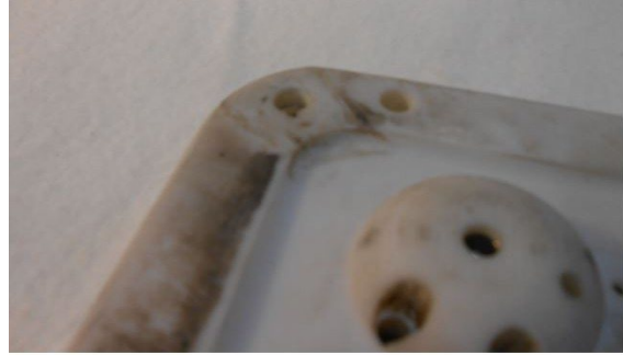
Figure 41. Chipping around the ceramic mold mounting hole.
